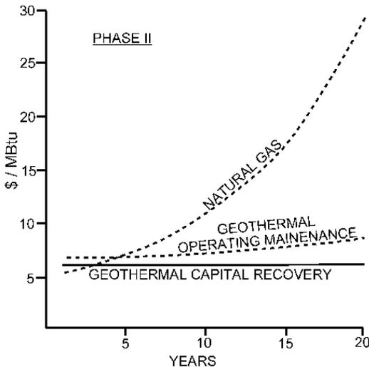
Figure 2. Phase II Unit Energy Cost Comparison (Lienau, 1981)
