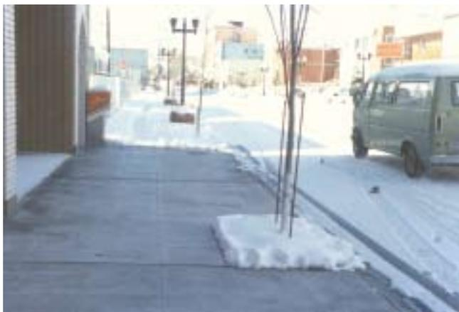
*Photo 4: Geothermally Heated Sidewalk Snowmelt (Geo-Heat Center)*
