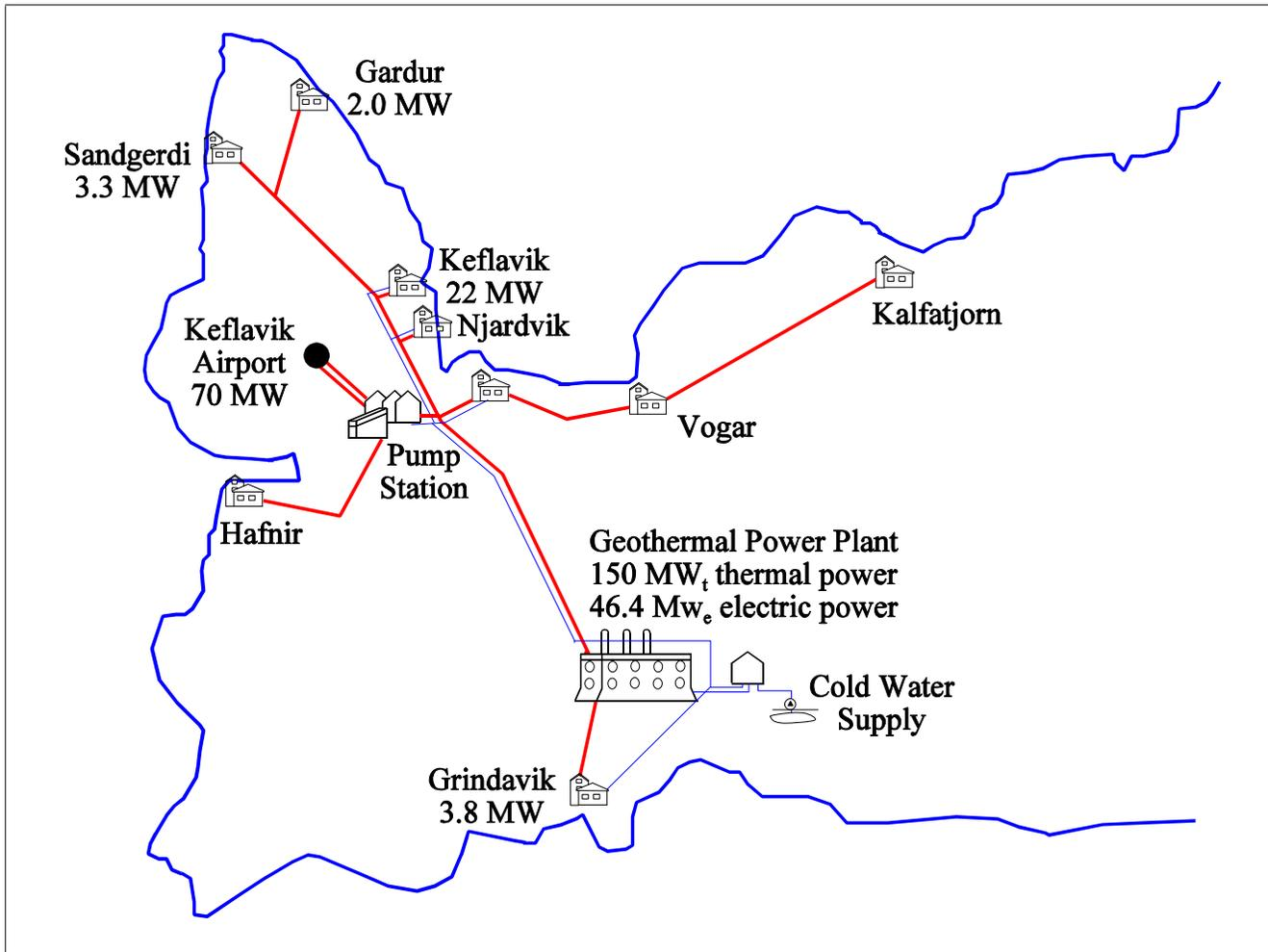
Figure 2. The Sudurnes Regional Heating System layout.
