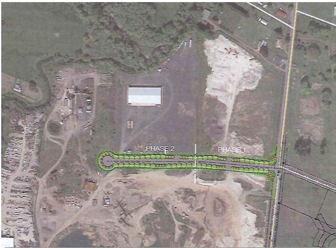
Figure 13. Satellite view indicating planned access road. Phase 1 to be a temporary road built by the seller.
