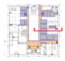
building by providing a single, level corridor access to all spaces. New restrooms will be accessible and the inaccessible second floor space is eliminated. The existing ramp system in the middle of the East wing is proposed to be eliminated. A single ramp at the north end of the East Wing provides access to two class/lab spaces that are not on the main level. The second level Campus Security space is relocated on the ground floor in the East Wing along with EH&S offices.
