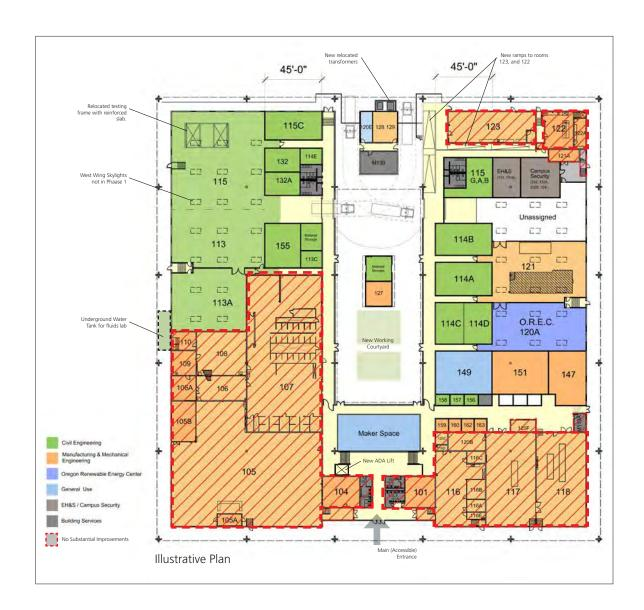
phase the southwest corner of the building will be substantially reconfigured to reuse the welding area (107) and rooms 106, 108, 109 and 110. This area will also provide a new circulation corridor to the new building (illustrated in Project 2).
