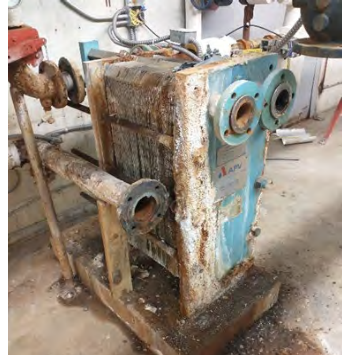
Sept. 2022- Corroded and failed building heat exchanger unit causing temporary building closure.
