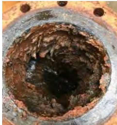
Spring 2022- Corroded and compromised Well #1.
